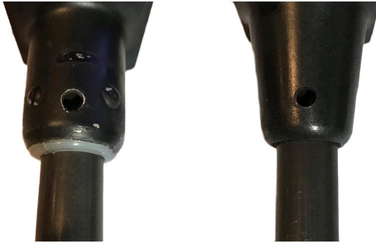
Figure 4. Yoke Collar Supports found on older Cessna 150's and 172's (Left), and 1971 and newer Cessna 150's, 152's and 172's (Right). See Appendix B for compatibility
