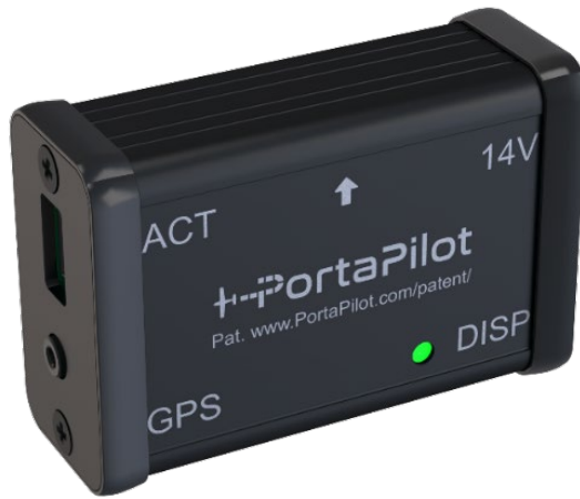
Figure 5. Orientation of the CM with arrow pointing up and facing the pilot.
