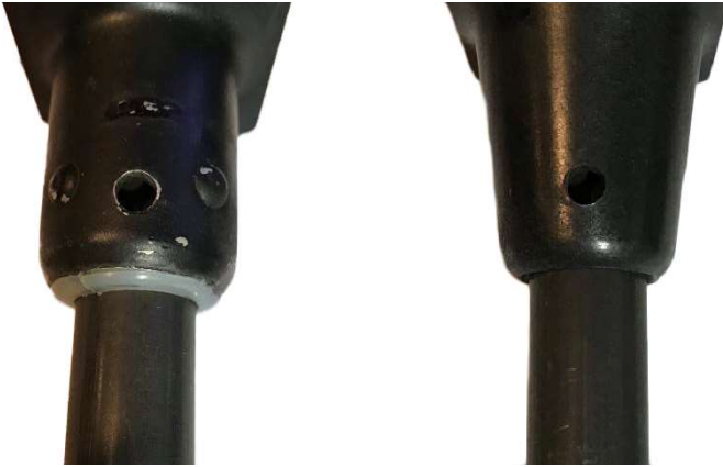
Figure 4. Yoke Collar Supports found on older Cessna 172's (Left), and 1971 and newer Cessna 172's (Right). See Appendix B for compatibility
