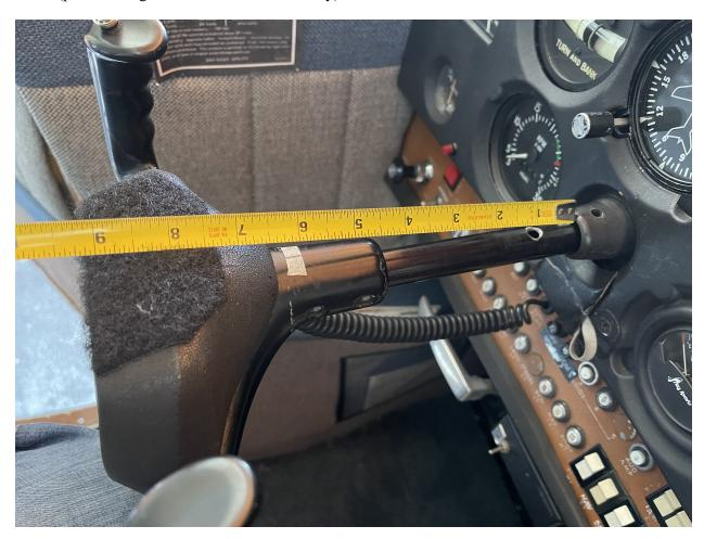
Refer to the table below to determine if a spacer is required. Match the extension amount that you measure to the nearest value in the table below. Spacer kits must be purchased separately. and comes with a spacer and three fasteners. The spacer must be placed between the top half of the Yoke Clamp and the Fork, using a small amount of blue loc-tite or similar on the fasteners.
